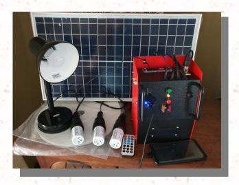
The Smart Units, produced locally by Tundra Energy, have a micro-processor, GPS, GSM and Bluetooth installed which allows for pre-paid or rental options to be considered. Working with local partners, Malawi Volunteer Organisation and Rift Valley Solar, we are hoping to determine the appeal of pre-paid / rental solar lighting systems and which rent to own option generates the best Return on Investment (ROI).
